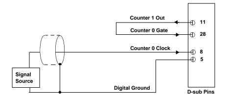
Figure 14: Connecting Counter/Timer Signals to the D-sub Pins for a Frequency Measurement Operation Using an External Pulse
