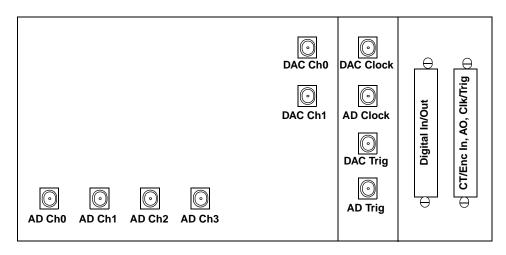
Figure 5: DT9832-04-2-BNC Version of the BNC Connection Box
