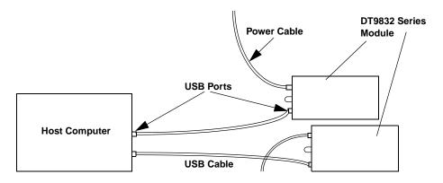
Figure 3: Attaching the Module to the Host Computer
