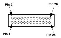
Figure 28: Orientation of the Pins for Connectors J1 on the EP353 Panel
