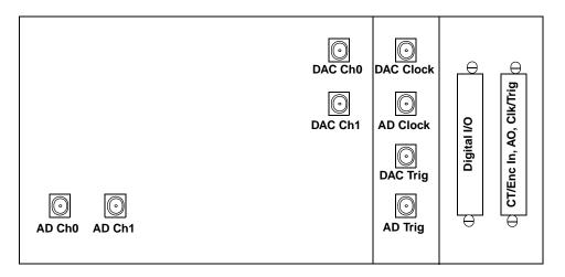
Figure 6: DT9832A-02-2-BNC Version of the BNC Connection Box
