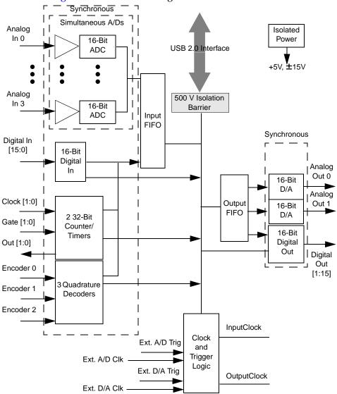
Figure 19 shows a block diagram of the DT9832 Series modules.
