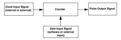
Figure 21: Counter/Timer Channel
