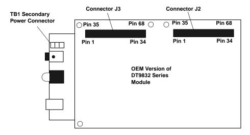
Figure 24: Connectors on OEM Version of DT9832 Module
