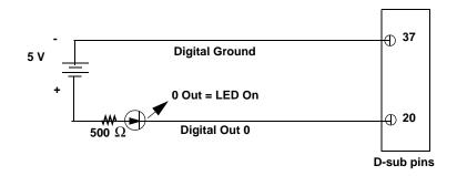
Figure 10: Connecting Digital Outputs to the D-sub Pins
