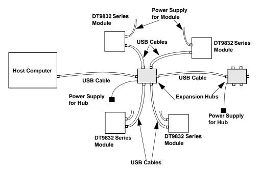
Figure 4: Attaching Multiple Modules Using Expansion Hubs
