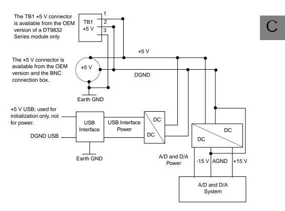
Figure 33: Ground, Power, and Isolation Connections
