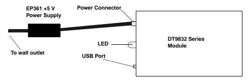
Figure 2: Attaching a +5 V Power Supply to the DT9832 Series Module
