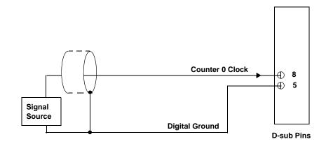
Figure 15: Connecting Counter/Timer Signals to the D-sub Pins for a Period/Pulse Width Measurement Operation
