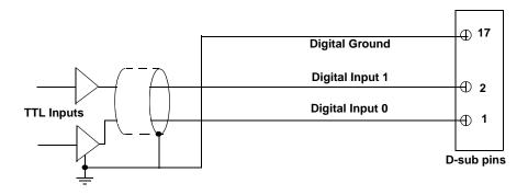
Figure 9: Connecting Digital Inputs to the D-sub Pins
