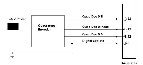
Figure 18: Connecting Quadrature Decoder Signals to the D-sub Pins
