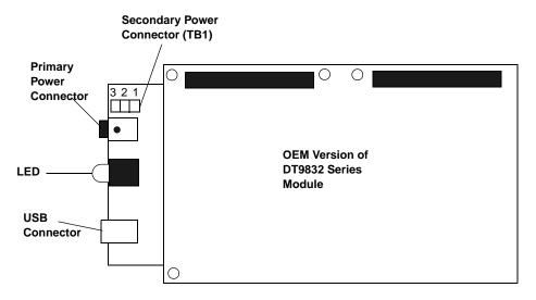
Figure 32: Secondary Power Connector
