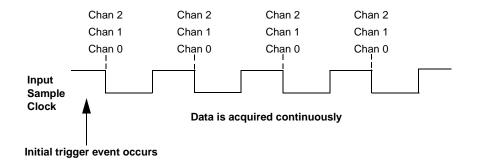
Figure 20: Continuous Scan Mode
