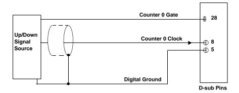
Figure 13: Connecting Counter/Timer Signals to the D-sub Pins for an Up/Down Counting Operation
