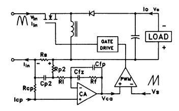
Fig. 11 - Flyback Preregulator Circuit
