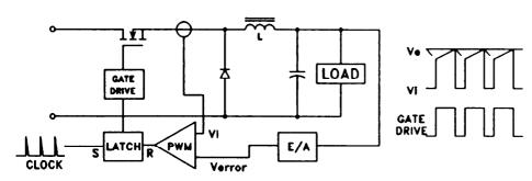
Fig. 1 - Peak Current Mode Control Circuit and Waveforms
