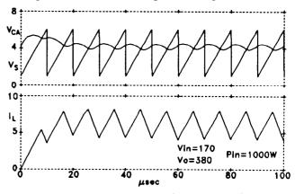
Fig. 7 - Boost Regulator Waveforms
