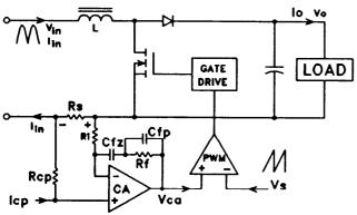
Fig. 6 - Boost Freregulator Circuit
