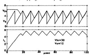
Fig. 3 - Buck Waveforms, Optimized Gain
