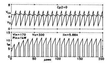
Fig. 12 - Flyback Regulator Waveforms
