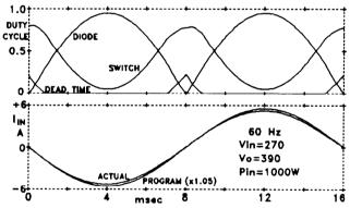
Fig. 9 - Boost 60Hz Sine Wave Input Current
