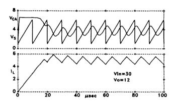
Fig. 4 - Buck with Additional Pole at  $f_s$
