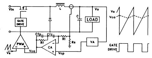
Fig. 2 - Average Current Mode Control Circuit and Waveforms
