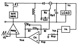
Fig. 14 - Flyback Output Current Control
