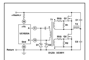
Low power transformers can be driven by the UC1525A. Automatic reset occurs during dead time, when both ends of the primary winding are switched to ground.
