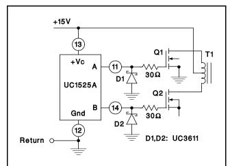
The low source impedance of the output drivers provides rapid charging of power FET Input capacitance while minimizing external components.
