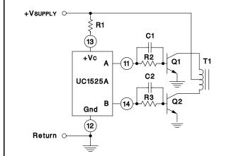
In conventional push-pull bipolar designs, forward base drive is controlled by R1-R3. Rapid turn-off times for the power devices are achieved with speed-up capacitors C1 and C2.
