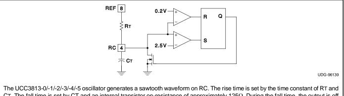
The UCC3813-0/-1/-2/-3/-4/-5 oscillator generates a sawtooth waveform on RC. The rise time is set by the time constant of RT and CT. The fall time is set by CT and an internal transistor on-resistance of approximately  $125\Omega$ . During the fall time, the output is off and the maximum duty cycle is reduced below 50% or 100% depending on the part number. Larger timing capacitors increase the discharge time and reduce the maximum duty cycle and frequency.
