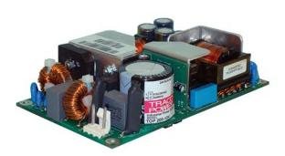
The new TOP-200 Series AC/DC Power Supplies feature the highest power rating in the industry standard  $3.0'' \times 5.0''$  (76.2 × 127 mm) footprint. They can supply up to 200 W output power with convection cooling over an industrial operating temperature range of -25°C to +70°C. This performance could be realized by a state of the art design providing an extremely high efficiency of >90 % which eliminates the need for a dedicated power supply cooling fan.
