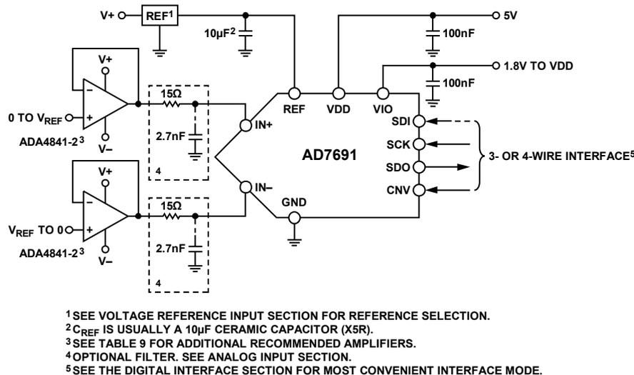
Figure 29. Typical Application Diagram with Multiple Supplies
