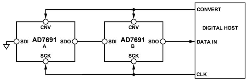
Figure 43. Chain Mode Without Busy Indicator Connection Diagram
