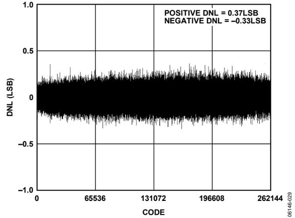
Figure 10. Differential Nonlinearity vs. Code, 5 V
