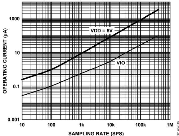
Figure 33. Operating Current vs. Sample Rate
