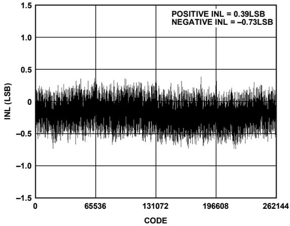
Figure 7. Integral Nonlinearity vs. Code 2.5 V
