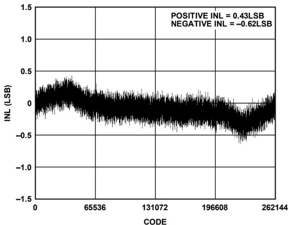
Figure 1. Integral Nonlinearity vs. Code, 5 V
