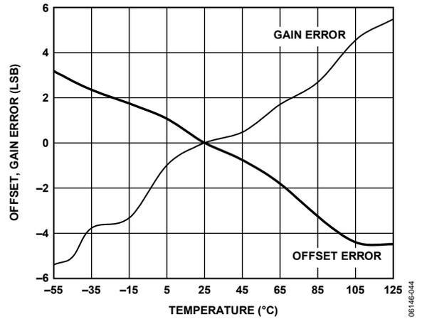
Figure 22. Zero Error, Gain Error vs. Temperature
