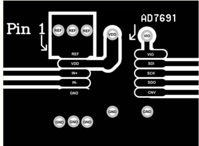
Figure 47. Example Layout of the AD7691 (Top Layer)
