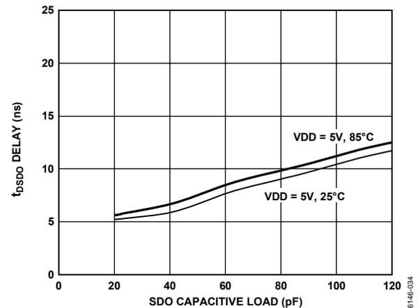
Figure 24.  $t_{\psi_{SDO}}$  Delay vs. Capacitance Load and Supply
