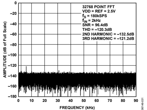
Figure 12. 2 kHz FFT Plot, 2.5 V
