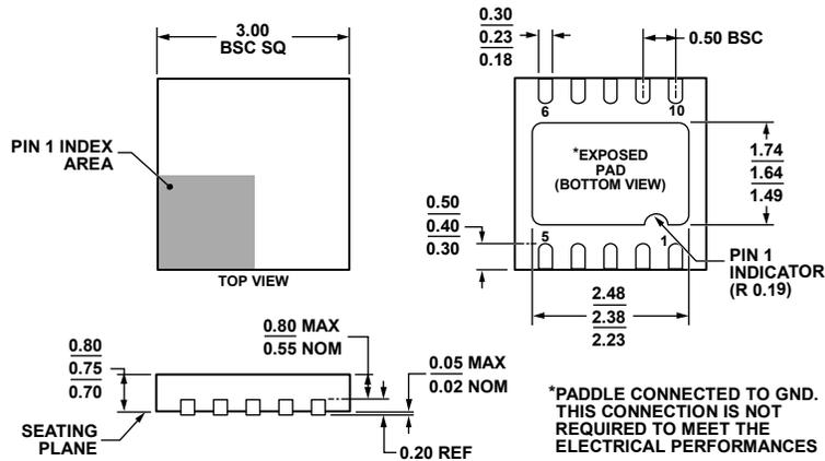
Figure 50. 10-Lead Lead Frame Chip Scale Package [QFN (LFCSP\_WD)]
