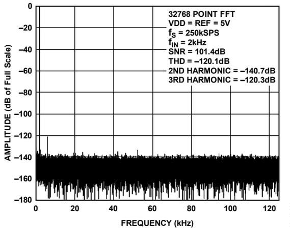
Figure 9. 2 kHz FFT Plot, 5 V
