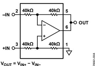
Figure 38. Difference Amplifier, Gain = 1
