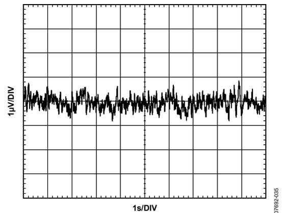
Figure 34. 0.1 Hz to 10 Hz Voltage Noise
