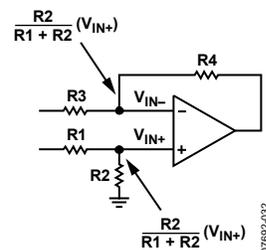
Figure 36. Voltage Division in the Difference Amplifier Configuration
