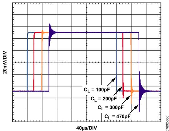
Figure 31. Small-Signal Step Response for Various Capacitive Loads
