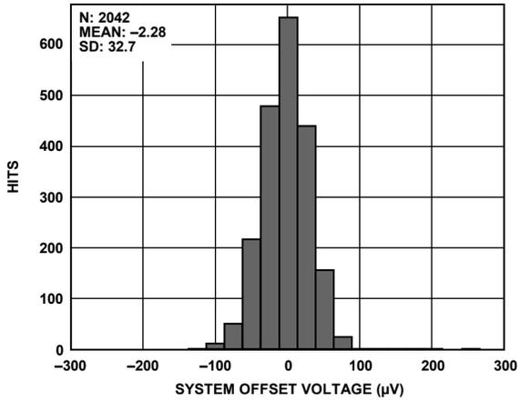
Figure 5. Distribution of Typical System Offset Voltage
