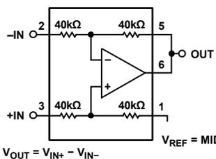
Figure 39. Difference Amplifier, Gain = 1, Referenced to Midsupply
