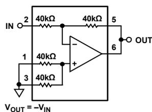
Figure 40. Inverting Amplifier, Gain = -1
