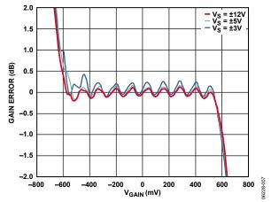
Figure 7. Gain Error vs.  $V_{GAIN}$  for Three Values of Supply Voltage (V<sub>s</sub>) (See Figure 56)
