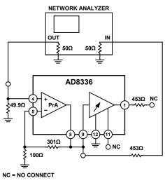
Figure 58. Frequency Response of the Preamp
