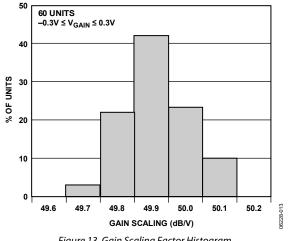
Figure 13. Gain Scaling Factor Histogram
