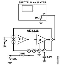
Figure 72. Input-Referred Noise vs. Source Resistance
