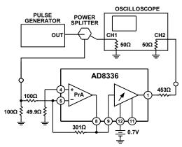
Figure 70. Pulse Response, Inverting Gain
