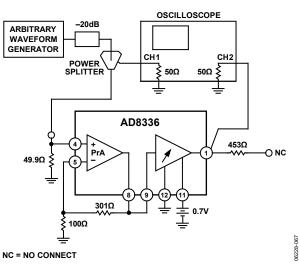
Figure 67. VGA Overdrive Recovery
