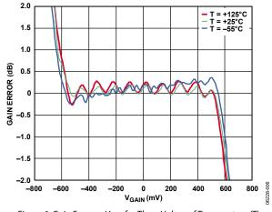
Figure 6. Gain Error vs. V<sub>GAIN</sub> for Three Values of Temperature (T) (See Figure 56)
