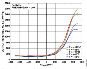
Figure 29. Output-Referred Noise vs. V<sub>GAIN</sub> at Various Temperatures (T) When the Preamp Gain is 20× (See Figure 62)
