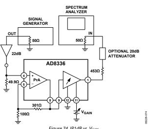
Figure 74. IP1dB vs. V<sub>GAIN</sub>
