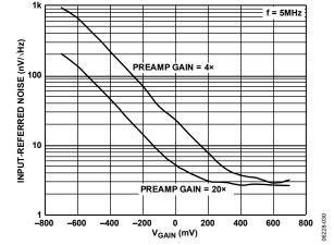
Figure 30. Input-Referred Noise vs. V<sub>GAIN</sub> for Preamp Gains of 4× and 20× (See Figure 62)
