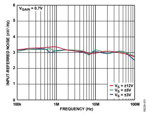
Figure 31. Short-Circuit Input-Referred Noise vs. Frequency at Maximum Gain for Three Values of Power Supply Voltage (V<sub>s</sub>) (See Figure 62)
