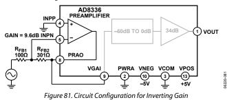
The considerations regarding total resistance vs. distortion, noise, and power that were noted in the noninverting case also apply in the inverting case, except that the amplifier can be operated at unity inverting gain. The signal gain is reduced while the noise gain is the same as for the noninverting configuration:
