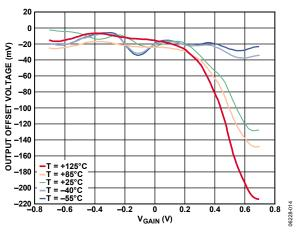
Figure 14. Output Offset Voltage vs. V<sub>GAIN</sub> for Various Values of Temperature (T)
