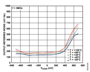
Figure 28. Output-Referred Noise vs. V<sub>GAIN</sub> at Various Temperatures (T) (See Figure 62)
