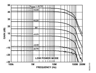
Figure 19. Frequency Response for Various Values of V<sub>GAIN</sub>, Low Power Mode (See Figure 57)
