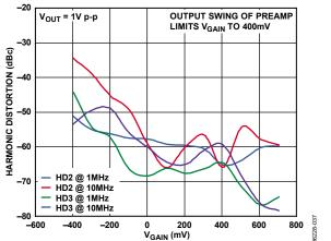
Figure 37. Second and Third Harmonic Distortion vs. V<sub>GAIN</sub> at 1 MHz and 10 MHz (See Figure 64)
