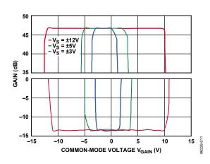
Figure 11. Gain vs. Common-Mode Voltage at  $V_{GAIN}$
