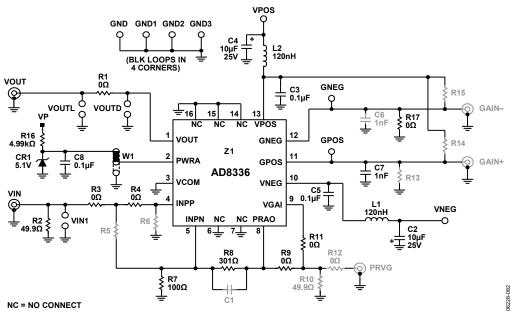
Figure 89. AD8336-EVALZ Schematic Shown as Shipped, Configured for a Noninverting Gain of  $4 \times$
