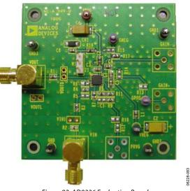
Figure 82. AD8336 Evaluation Board
