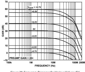
Figure 20. Frequency Response for Various Values of V<sub>GAIN</sub> When the Preamp Gain is 20× (See Figure 57)
