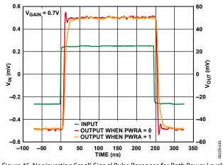
Figure 45. Noninverting Small-Signal Pulse Response for Both Power Levels (See Figure 65)
