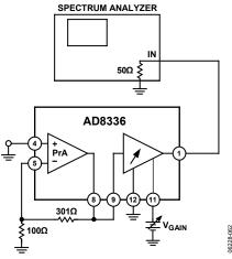
Figure 62. Input-Referred Noise and Output-Referred Noise
