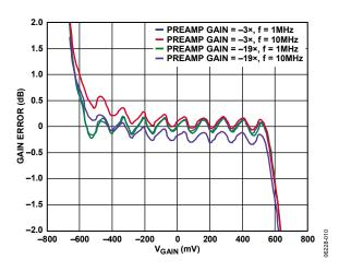
Figure 10. Gain Error vs. V<sub>GMN</sub> at 1 MHz and 10 MHz and for Inverting Preamp Gains of −3× and −19× (See Figure 56)
