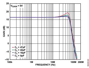
Figure 22. Frequency Response for Various Values of Load Capacitance (C<sub>L</sub>) (See Figure 57)
