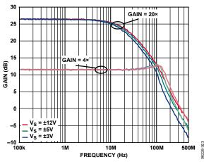
Figure 23. Preamp Frequency Response for Three Values of Supply Voltage (Vs) When the Preamp Gain is 4× or 20× (See Figure 58)
