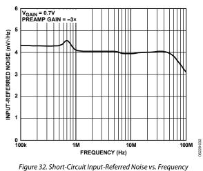
igure 32. Short-Circuit Input-Referred Noise vs. Frequenc at Maximum Inverting Gain (See Figure 73)
