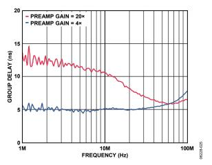
Figure 25. Group Delay vs. Frequency for Preamp Gains of 4× and 20× (See Figure 59)
