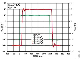
Figure 49. Large-Signal Pulse Response for Various Values of Load Capacitance Using ±3 V Power Supplies (See Figure 65)
