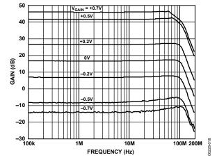
Figure 18. Frequency Response for Various Values of V<sub>GAIN</sub> (See Figure 57)
