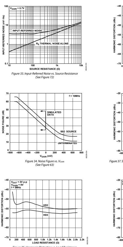
Figure 35. Harmonic Distortion vs. Load Resistance (See Figure 64)
