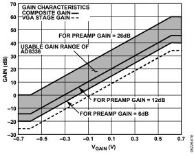
Figure 78. Ideal Gain Characteristics of the AD8336
