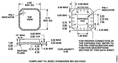
Figure 90. 16-Lead Lead Frame Chip Scale Package [LFCSP\_VQ] 4 mm × 4 mm Body, Very Thin Quad (CP-16-4) Dimensions shown in millimeters
