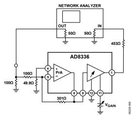
Figure 69. Frequency Response, Inverting Gain
