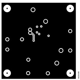
Figure 85. Secondary Side Copper
