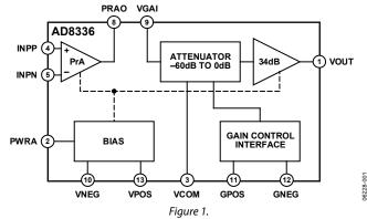
The large supply voltage range makes the AD8336 particularly suited for industrial medical applications and for video circuits. Dual-supply operation enables bipolar input signals, such as those generated by photodiodes or photomultiplier tubes.
