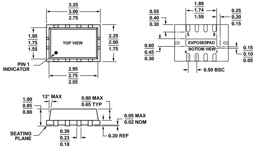
Figure 43. 8-Lead Lead Frame Chip Scale Package [LFCSP\_VD]
