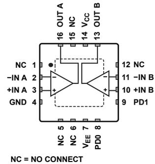
Figure 1. Thermally Enhanced, 4 mm × 4 mm, 16-Lead LFCSP\_WQ
