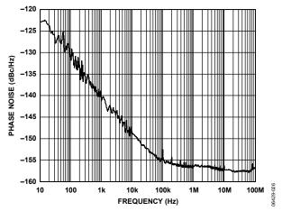
Figure 20. Phase Noise (Additive) LVPECL @ 245.76 MHz, Divide-by-1
