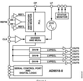
The AD9518-0 features six LVPECL outputs (in three pairs). The LVPECL outputs operate to 1.6 GHz.
