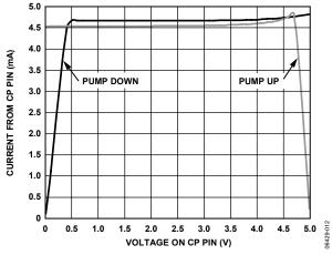
Figure 8. Charge Pump Characteristics @  $V_{CP} = 5.0 \text{ V}$
