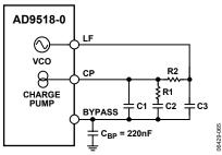
Figure 31. Example of External Loop Filter for PLL
