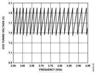
Figure 11. VCO Tuning Voltage vs. Frequency
