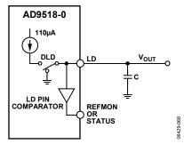
Figure 34. Current Source Lock Detect
