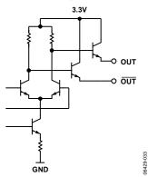
Figure 41. LVPECL Output Simplified Equivalent Circuit
