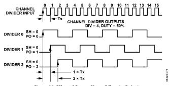
Figure 38. Effect of Coarse Phase Offset (or Delay)
