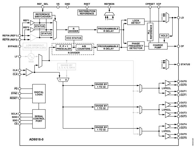
Figure 29. Clock Distribution or External VCO < 1600 MHz
