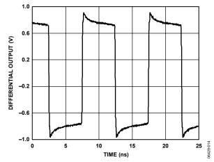
Figure 14. LVPECL Output (Differential) @ 100 MHz
