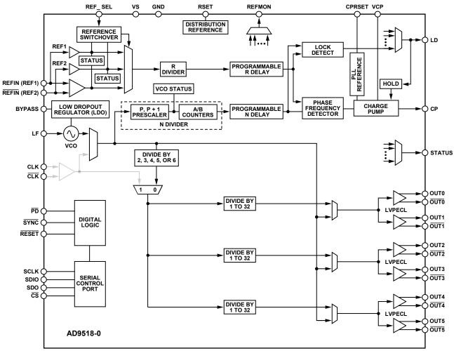
Figure 28. Internal VCO and Clock Distribution
