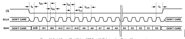
Figure 46. Serial Control Port Write—MSB First, 16-Bit Instruction, Timing Measurements
