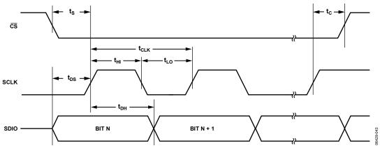
Figure 49. Serial Control Port Timing—Write
