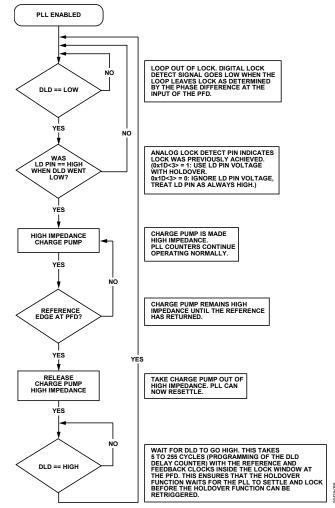
Figure 36. Flow Cchart of Automatic/Internal Holdover Mode
