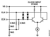
Figure 35. CLK Equivalent Input Circuit
