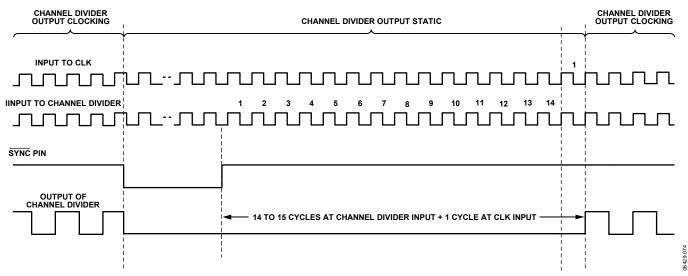
Figure 40. SYNC Timing when VCO Divider Is Not Used—CLK Input Only
