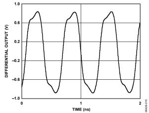
Figure 15. LVPECL Output (Differential) @ 1600 MHz
