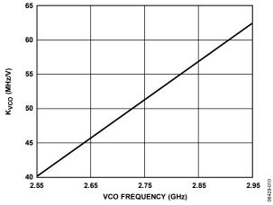
Figure 6. VCO K<sub>VCO</sub> vs. Frequency
