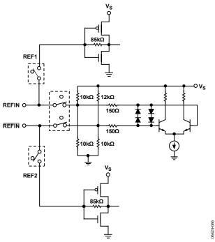
Figure 32. REFIN Equivalent Circuit
