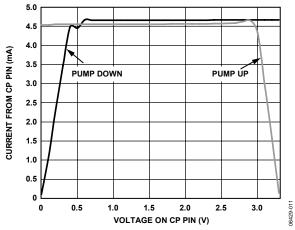
Figure 7. Charge Pump Characteristics @  $V_{CP} = 3.3 \text{ V}$
