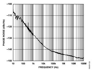
Figure 22. Phase Noise (Additive) LVPECL @ 1600 MHz, Divide-by-1
