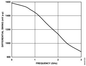
Figure 16. LVPECL Differential Swing vs. Frequency
