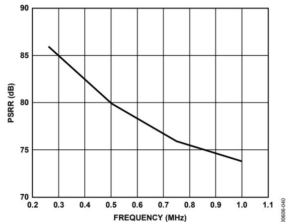
Figure 41. AVDD Power Supply Rejection Ratio vs. Frequency
