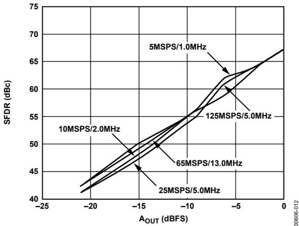
Figure 11. Single-Tone SFDR vs.  $A_{OUT}$  @  $f_{OUT} = f_{CLK}/5$
