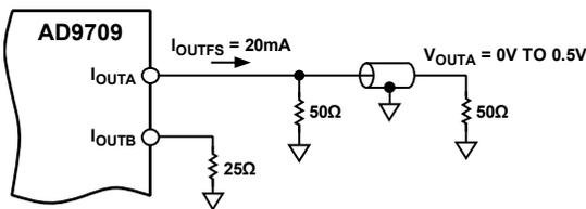
Figure 39. 0 V to 0.5 V Unbuffered Voltage Output
