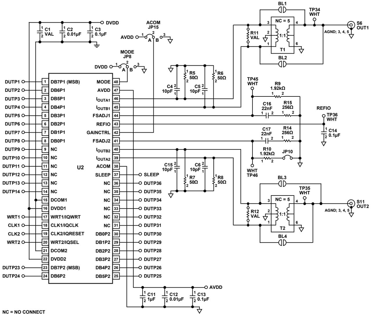
Figure 48. AD9709 and Output Signal Conditioning
