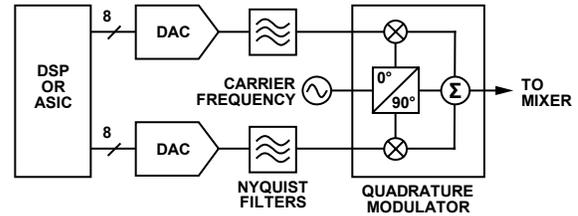
Figure 43. Typical Analog QAM Architecture
