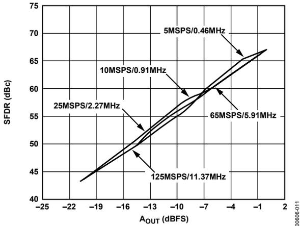
Figure 10. Single-Tone SFDR vs.  $A_{OUT}$  @  $f_{OUT} = f_{CLK}/11$
