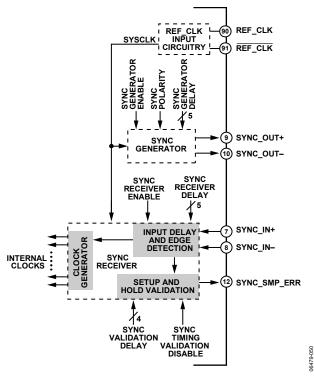
Figure 50. Synchronization Circuit Block Diagram
