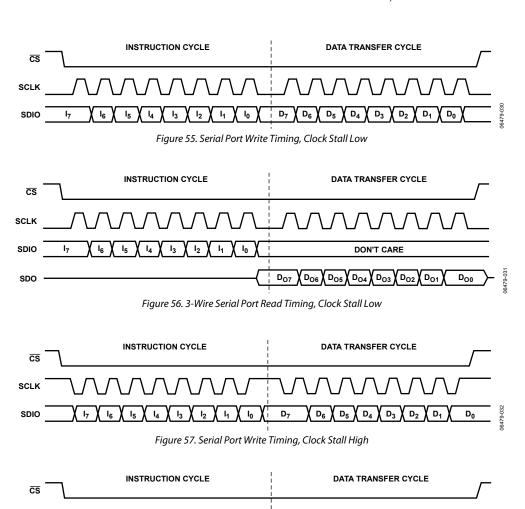
Figure 58. 2-Wire Serial Port Read Timing, Clock Stall High
