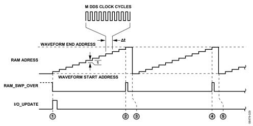
Figure 48. Continuous Recirculate Timing Diagram
