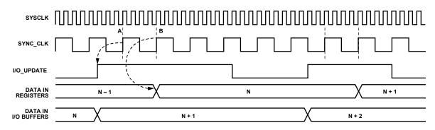
THE DEVICE REGISTERS AN I/O UPDATE AT POINT A. THE DATA IS TRANSFERRED FROM THE ASYNCHRONOUSLY LOADED I/O BUFFERS AT POINT B. Figure 49. I/O\_UPDATE Transferring Data from I/O Buffer to Active Registers
