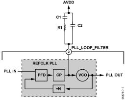
Figure 35. REFCLK PLL External Loop Filter
