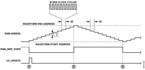
Figure 47. Continuous Bidirectional Ramp Timing Diagram
