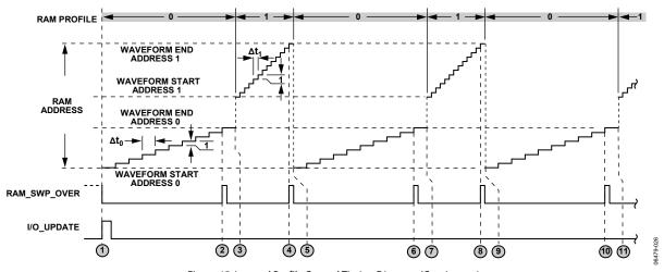
Figure 45. Internal Profile Control Timing Diagram (Continuous)
