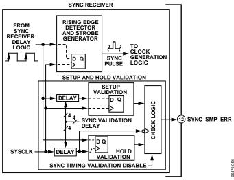
Figure 54. Sync Timing Validation Block
