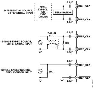
Figure 32. Direct Connection Diagram
