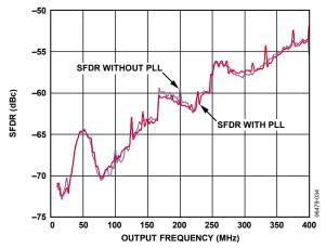
Figure 6. Wideband SFDR vs. Output Frequency (PLL with Reference Clock = 15.625 MHz  $\times$  64)
