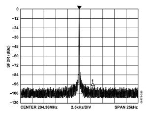
Figure 13. Narrow-Band SFDR at 204.36 MHz, REFCLK = 1 GHz
