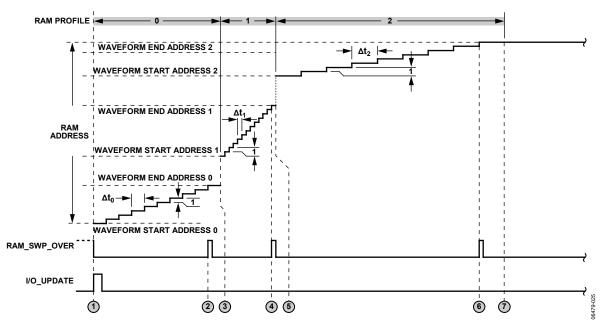
Figure 44. Internal Profile Control Timing Diagram (Burst)
