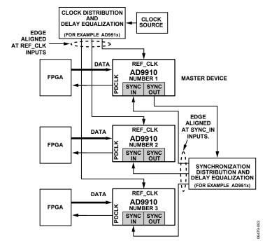
Figure 53. Multichip Synchronization Example
