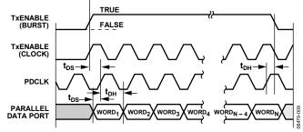
Figure 26. PDCLK and TxENABLE Timing Diagram
