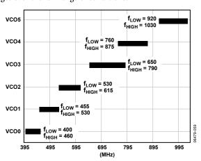
Figure 33. VCO Ranges Including Atypical Wafer Process Skew
