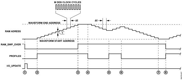
Figure 46. Bidirectional Ramp Timing Diagram
