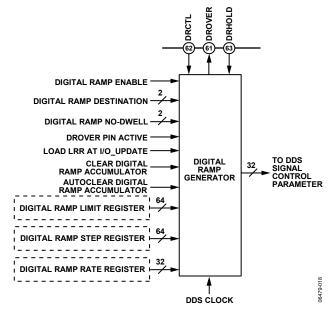
Figure 37. Digital Ramp Block Diagram
