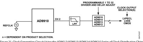
Figure 21. Clock Generation Circuit Using the AD9512/AD9513/AD9514/AD9515 Series of Clock Distribution Chips
