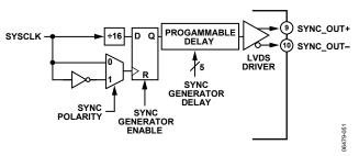
Figure 51. Sync Generator Diagram
