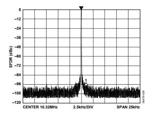
Figure 12. Narrow-Band SFDR at 10.32 MHz, REFCLK = 1 GHz
