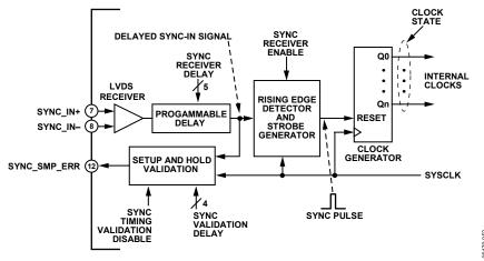
Figure 52. Sync Receiver Diagram
