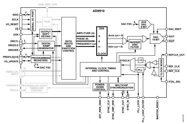
Figure 24. Digital Ramp Modulation Mode
