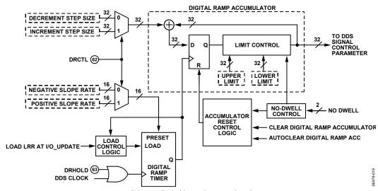
Figure 38. Digital Ramp Generator Detail
