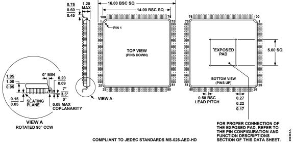
Figure 59. 100-Lead Thin Quad Flat Package, Exposed Pad [TQFP\_EP] (SV-100-4) Dimensions shown in millimeters
