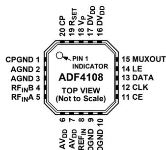
Figure 3. Pin Configuration
