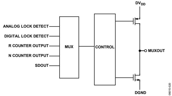
Figure 14. MUXOUT Circuit
