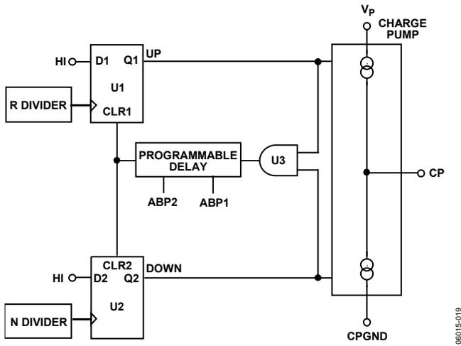
Figure 13. PFD Simplified Schematic and Timing (in Lock)
