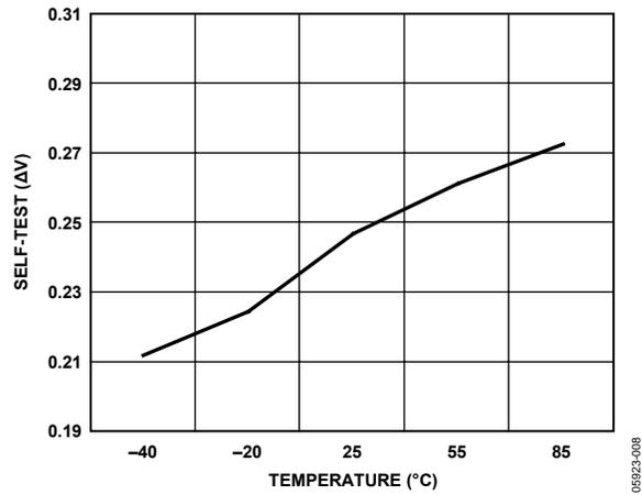
Figure 8. Self-Test vs. Temperature, VCC = 5 V
