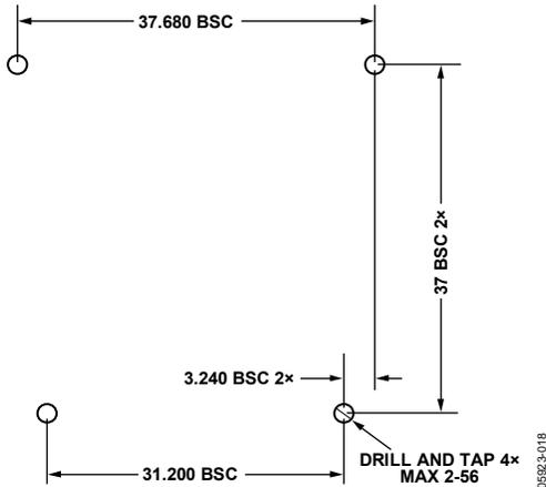
Figure 17. Bulkhead Mount Attachment Hole Locations
