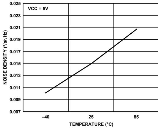
Figure 10. Noise Density vs. Temperature, VCC = 5 V
