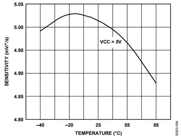
Figure 6. Gain Sensitivity vs. Temperature @ ±300°/sec
