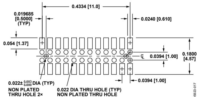
Figure 16. Mating Socket Recommended Pad Layout
