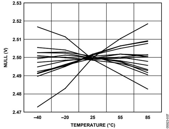
Figure 7. Null vs. Temperature, VCC = 5 V
