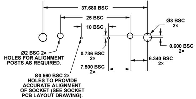
Figure 18. Interface Board Hole Locations for Bulkhead Mount
