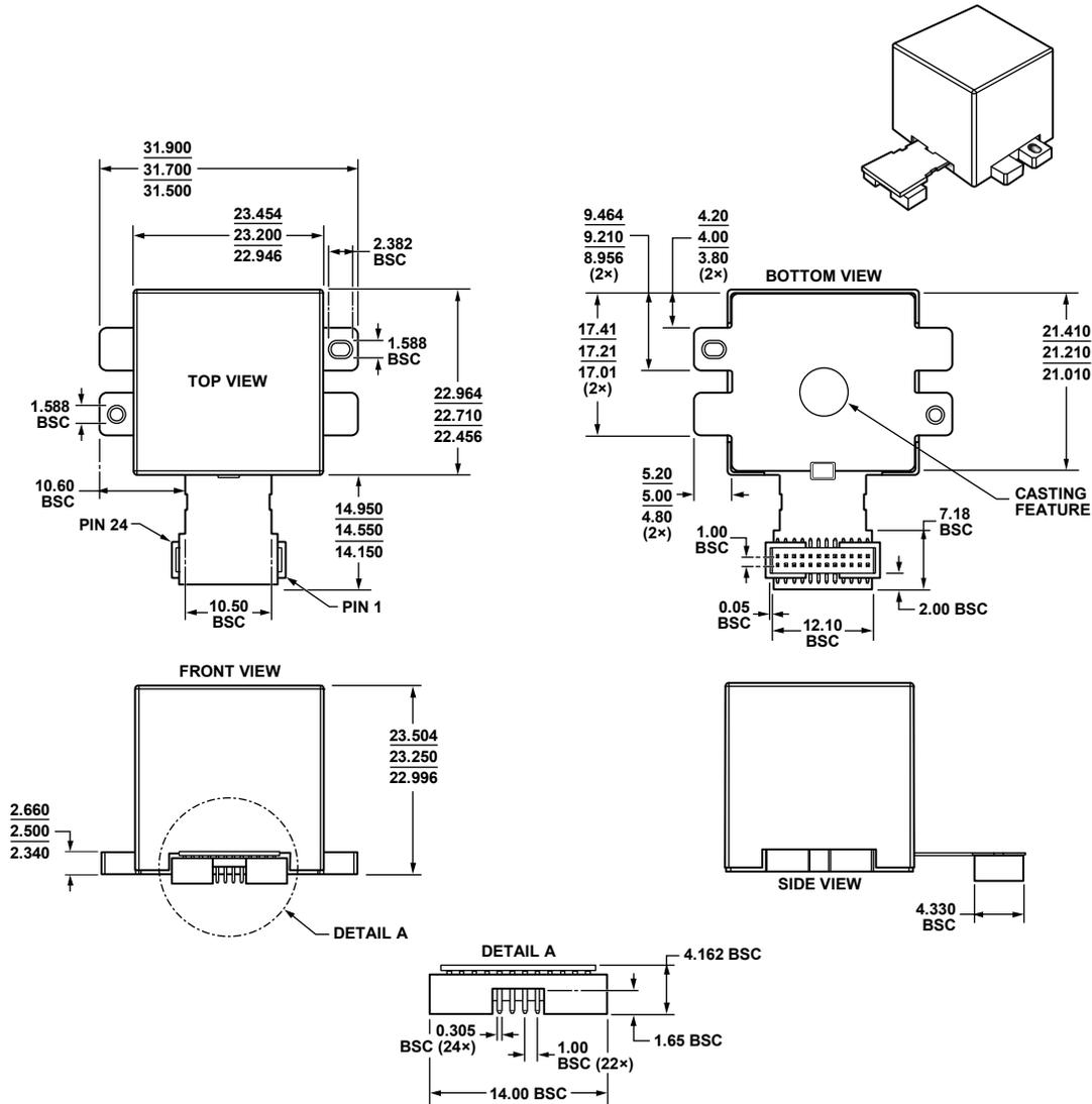
Figure 16. 24-Lead Module with Connector Interface
