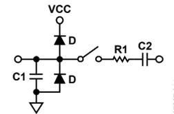
Figure 14. Equivalent Analog Input Circuit
