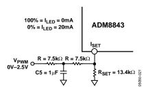
Figure 21. PWM Brightness Control Using Filter-PWM Signal
