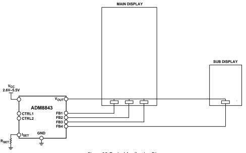
Figure 25. Typical Application Diagram
