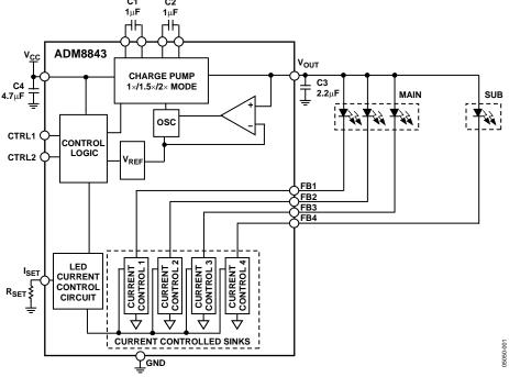
Figure 18. Functional Block Diagram
