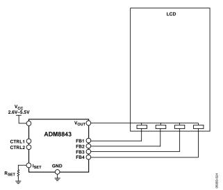
Figure 23. Driving Four White LEDs
