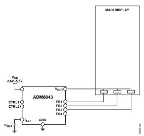
Figure 24. Driving Three White LEDs
