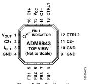
Figure 2. Pin Configuration
