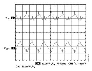
Figure 27. 1.5× Mode Operation, Four LEDs with 20 mA/LED at  $V_{CC}$  = 3.6 V, with a 1  $\mu$ F  $V_{CC}$  Decoupling Capacitor
