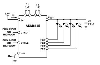
Figure 19. Digital PWM Brightness Control Application Diagram
