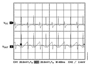
Figure 13. 2× Mode Operating Waveforms
