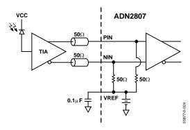
Figure 24. ADN2807 with DC-Coupled Inputs
