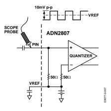
Figure 9. Single-Ended Sensitivity Measurement
