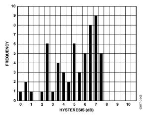
Figure 5. LOS Hysteresis OC-3,  $-40^{\circ}$ C, 3.6 V,  $2^{23}-1$  PRBS Input Pattern,  $R_{TH}=90~\text{k}\Omega$
