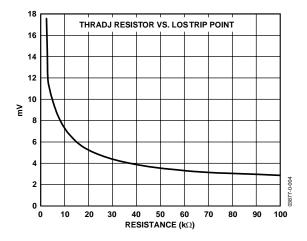
Figure 4. LOS Comparator Trip Point Programming
