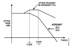
Figure 14. Jitter Response vs. Conventional PLL
