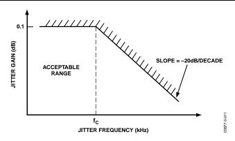
Figure 11. Jitter Transfer Curve
