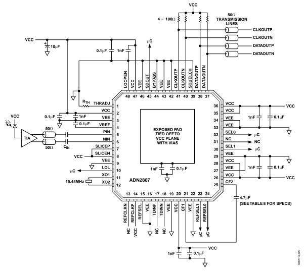
Figure 20. Typical Application Circuit
