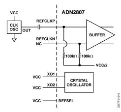
Figure 16. Single-Ended REFCLK Configuration
