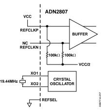
Figure 17. Crystal Oscillator Configuration
