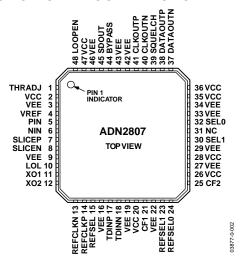
Figure 2. Pin Configuration
