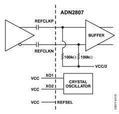
Figure 15. Differential REFCLK Configuration
