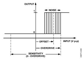
Figure 8. Input Sensitivity and Input Overdrive
