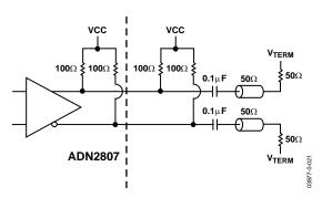
Figure 21. AC-Coupled Output Configuration
