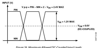
Figure 26. Maximum Allowed DC-Coupled Input Levels
