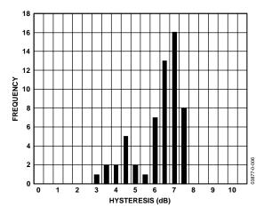
Figure 6. LOS Hysteresis OC-12,  $-40^{\circ}$ C, 3.6 V,  $2^{23}$  -1 PRBS Input Pattern,  $R_{TH} = 90 \text{ k}\Omega$
