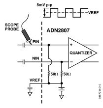
Figure 10. Differential Sensitivity Measurement
