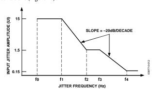
Figure 12. SONET Jitter Tolerance Mask
