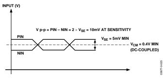
Figure 25. Minimum Allowed DC-Coupled Input Levels
