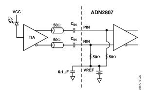
Figure 22. AC-Coupled Input Configuration
