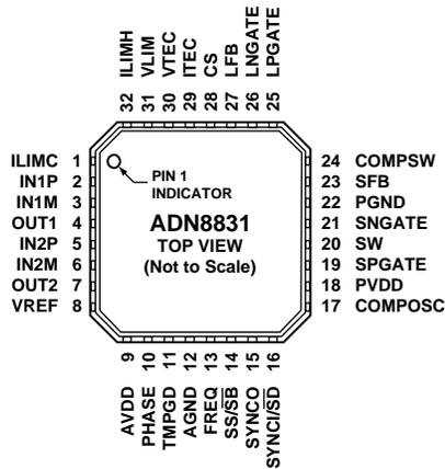
Figure 2. Pin Configuration
