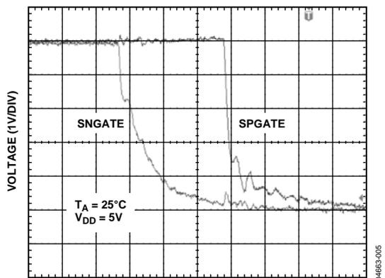
Figure 5. SNGATE and SPGATE Fall Time Using Circuit Shown in Figure 12
