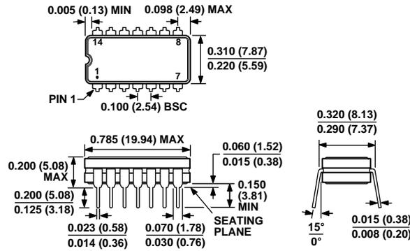
CONTROLLING DIMENSIONS ARE IN INCHES; MILLIMETER DIMENSIONS
