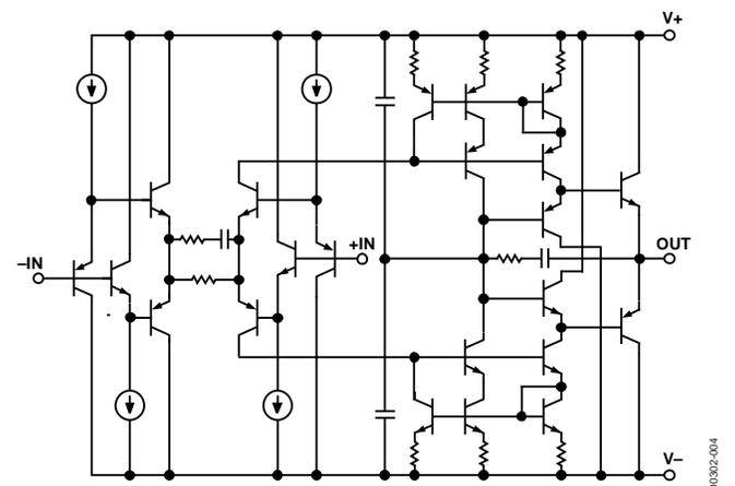
Figure 4. Simplified Schematic
