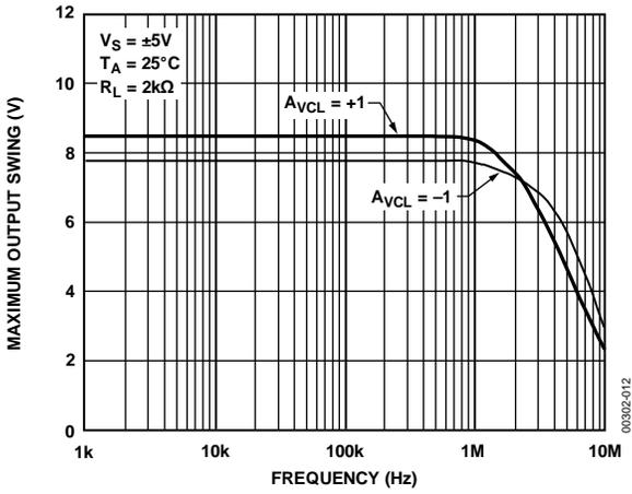
Figure 12. Maximum  $V_{OUT}$  Swing vs. Frequency
