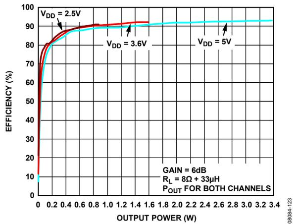
Figure 25. Efficiency vs. Output Power into  $8 \Omega$
