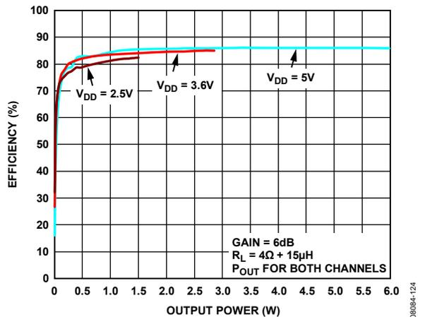
Figure 26. Efficiency vs. Output Power into  $4 \Omega$
