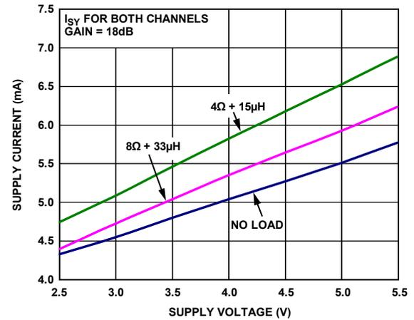
Figure 20. Supply Current vs. Supply Voltage,  $A_v = 18dB$
