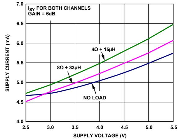
Figure 19. Supply Current vs. Supply Voltage,  $A_v = 6dB$
