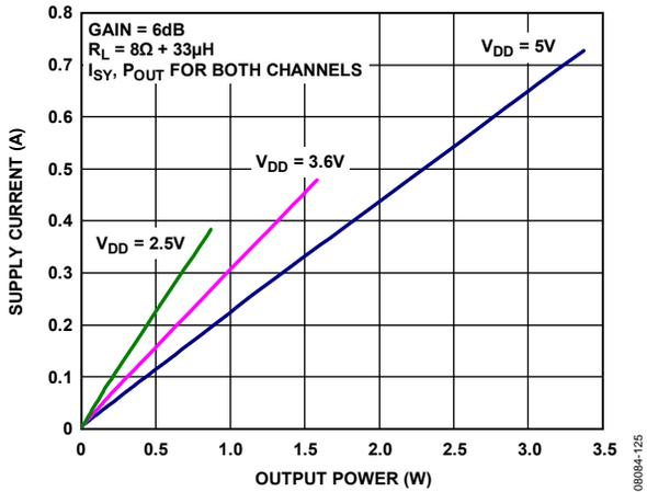
Figure 27. Supply Current vs. Output Power into 8  $\Omega$
