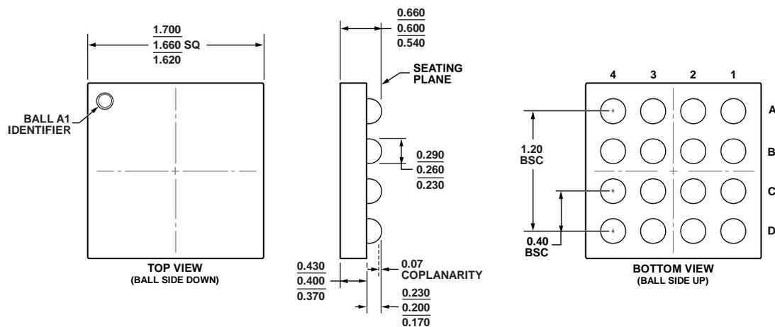
Figure 4. 16-Ball Wafer Level Chip Scale Package [WLCSP]
