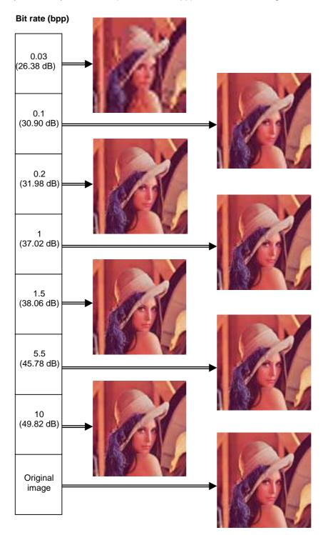
Figure 4 The reconstructed images based on several base layer bitstreams. (Numbers in the left column are in bpp.)
