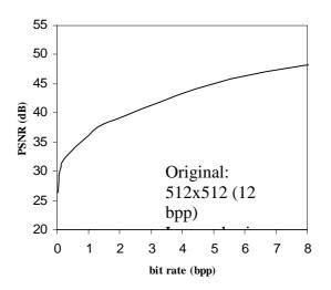
Figure 3. The compression performance of the CHC-RIOT base layer coder.
