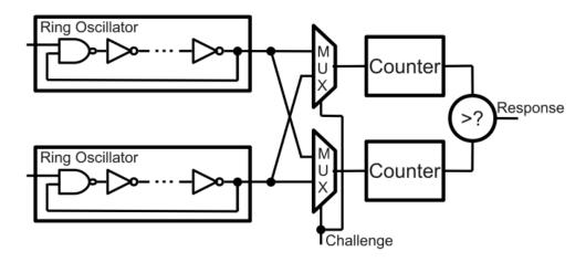
Figure 4.2. A 1-bit ring oscillator PUF
