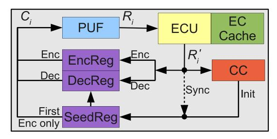
Figure 5.2. Block level view of a PUF ROK allowing out of order execution
