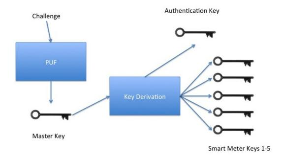
Figure 7.3. The key derivation process
