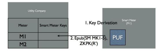
Figure 7.2. Storage of the derived keys
