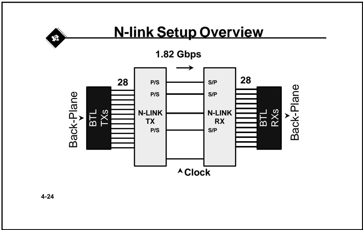
N-Link can provide multiple Gbps of throughput in any one direction. The above application can easily be replicated in the opposite direction to provide a full duplex solution running at 1.8 Gbps.
