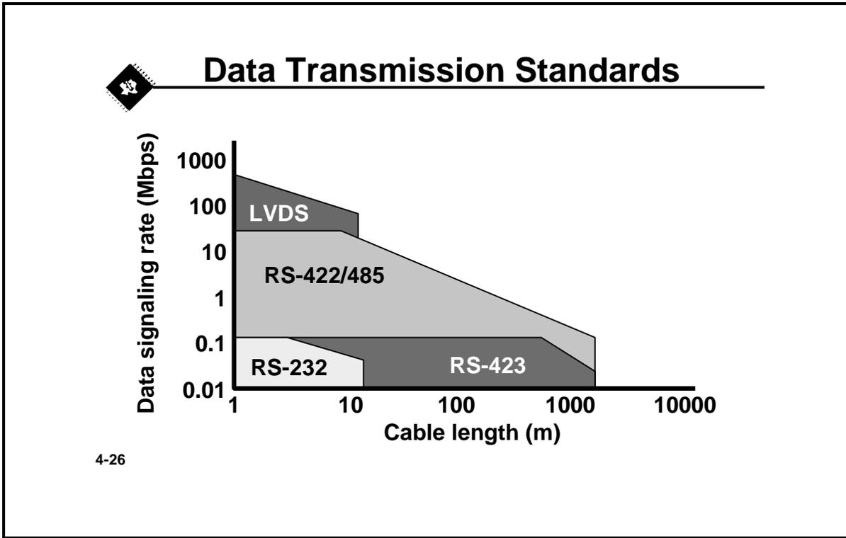
As shown in the beginning of this presentation, besides LVDS there are other standards which TI supports. TI has 30 years of experience in the Data Transmission arena; and it is therefore no wonder that along with its efforts to extend the data transmission capabilities of new technologies like LVDS, it also continues to improve currently implemented transmission specifications such as 232, 422, 485, and others.
