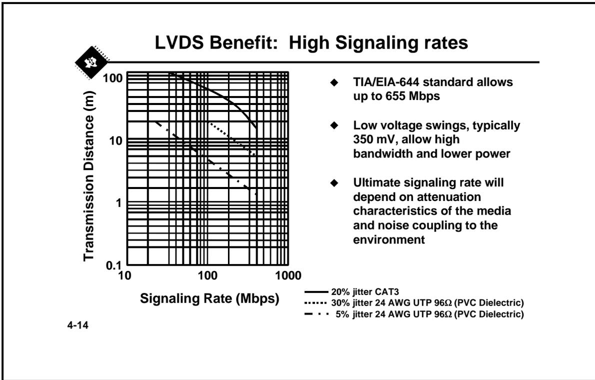
TIA/EIA-644 specifies drivers and receivers capable of operating at data signaling rates up to 655Mbps, and a theoretical maximum limit is calculated at 1.923 gbps. LVDS greatly exceeds the signaling rate capabilities of former differential standards like 485 and 422. And although PECL and ECL devices are also capable of high data rates, they can consume up to 10 times more the power than LVDS.
