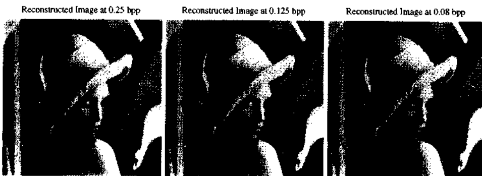
Figure 10.3: Reconstructed images for 32:1, 64:1, and 100:1 compression with (9, 7) filters.
