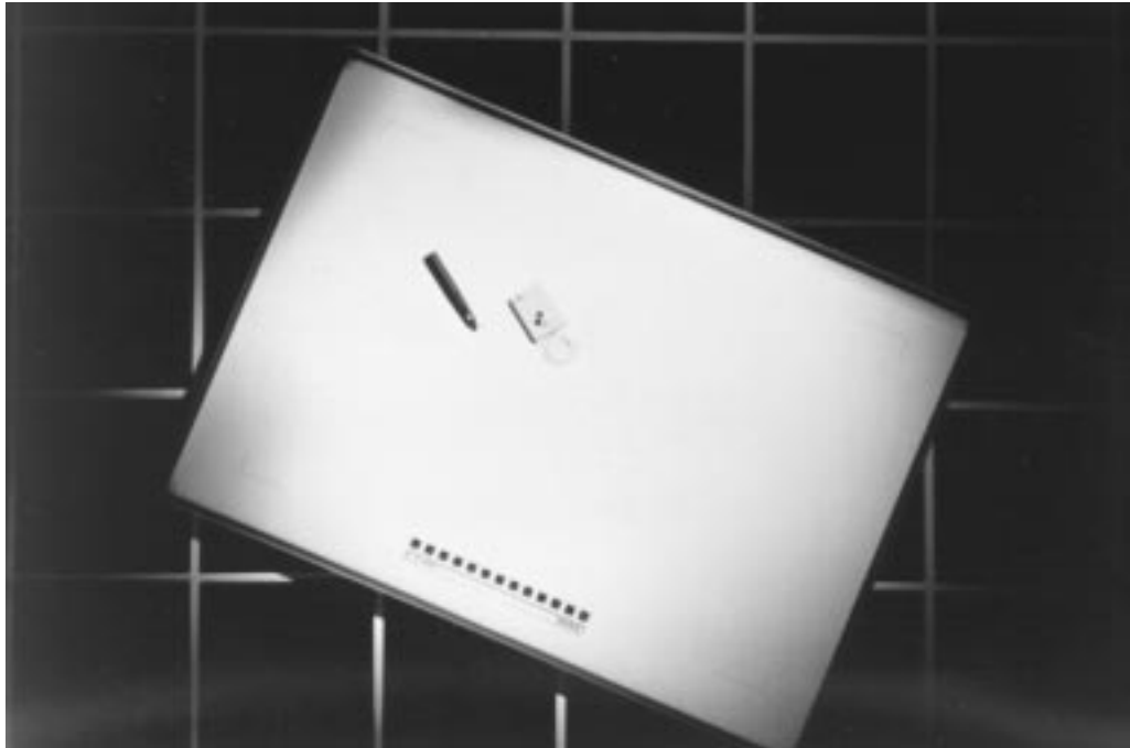
FIGURE 12.10 The popular pad digitizer includes a lightweight puck or pen-type pointer for selecting points whose coordinates are transmitted to a computer for processing.
