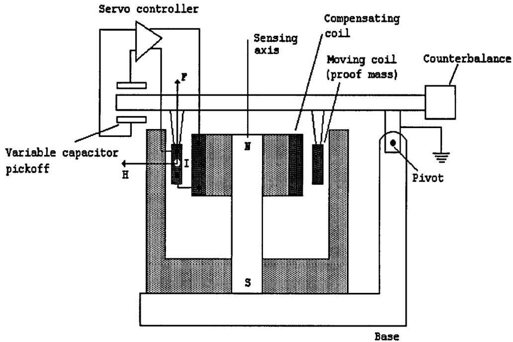
**FIGURE 17.6** A basic coil and permanent magnet accelerometer. The coil is supported by an arm with minimum friction bearings to form a proof mass in a magnetic field. Displacement of the coil due to acceleration induces an electric potential in the coil to be sensed and processed. A servo system maintains the coil in a null position.
