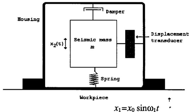
**FIGURE 17.1** A typical deflection-type seismic accelerometer. In this basic accelerometer, the seismic mass is suspended by a spring or cantilever inside a rigid frame. The frame is connected to the vibrating structure; as vibrations take place, the mass tends to remain fixed so that relative displacements can be picked up. They are manufactured in many different types and sizes and they exhibit diverse characteristics.
