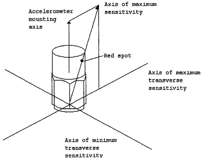
**FIGURE 17.19** Vectorial illustration of cross-axis sensitivity. Accelerometers may sense vibrations not only in the direction of main axis, but also perpendicular to the main axis. These cross-axis responses are minimized in many accelerometers to a value less than 1%. Sometimes, this sensitivity is used to determine the correct orientation of the device.
