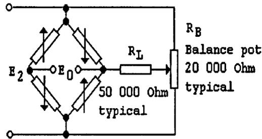
**FIGURE 17.21** Bridge circuit for piezoresistive and strain gage accelerometers. The strain gages form the four arms of the bridge. The two extra resistors are used for balancing and fine adjustment purposes. This type of arrangement reduces temperature effects.
