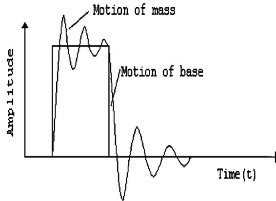
**FIGURE 17.3** Time response of a shock excitation of a single degree-of-freedom system. As the duration of the shock pulse increases, sustained oscillations get shorter in time but larger in amplitude. The maximum system response may be as high as twice the magnitude of the shock pulse.
