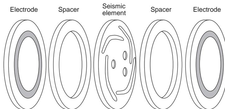
**FIGURE 17.12** Diaphragm-type capacitive accelerometer. The seismic element is cushioned between the electrodes. Motion of the mass between the electrodes causes air movement passing through the holes, which provides a squeeze film damping. In some cases, oil can be used as the damping element.
