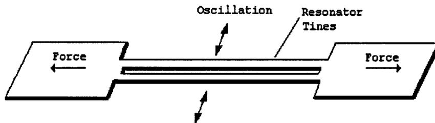
**FIGURE 17.18** A double-ended tuning fork (DETF) acceleration transducer. Two beams are vibrated  $180^\circ$  out of phase to eliminate reaction forces at the beam ends. The resonant frequency of the beam is altered by acceleration. The signal processing circuits are also integrated in the same chip.
