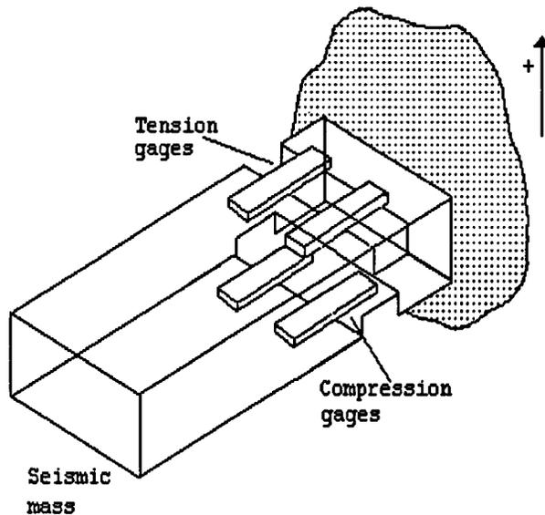
**FIGURE 17.10** Bonding of piezoelectric and piezoresistive elements onto an inertial system. As the inertial member vibrates, deformation of the tension and compression gages causes the resistance to change. The change in resistance is picked up and processed further. Accelerometers based on PZTs are particularly useful in medium- to high-frequency applications.
