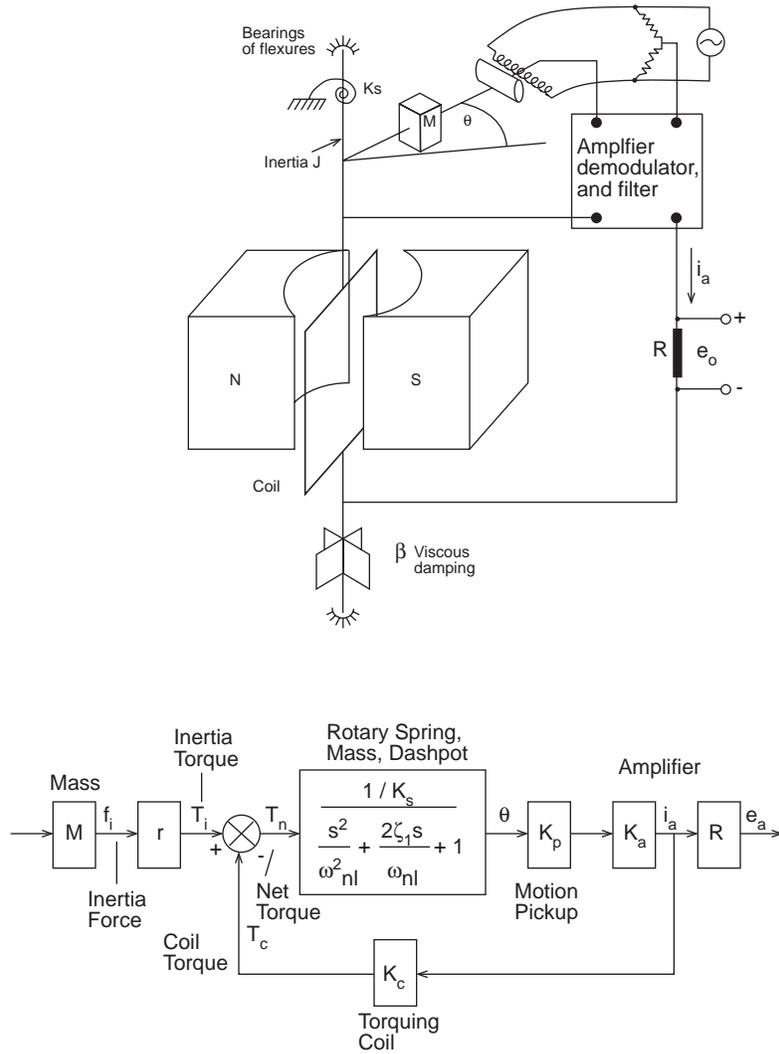
**FIGURE 17.7** A simplified version of a rotational type servo-accelerometer. Acceleration of the instrument case causes an inertial force on the sensitive mass, tending to make it pivot in its bearings or flexure mount. The rotation from neutral is sensed by inductive sensing and amplified, demodulated, and filtered to produce a current directly proportional to the motion from the null. The block diagram representation is useful in analysis.
