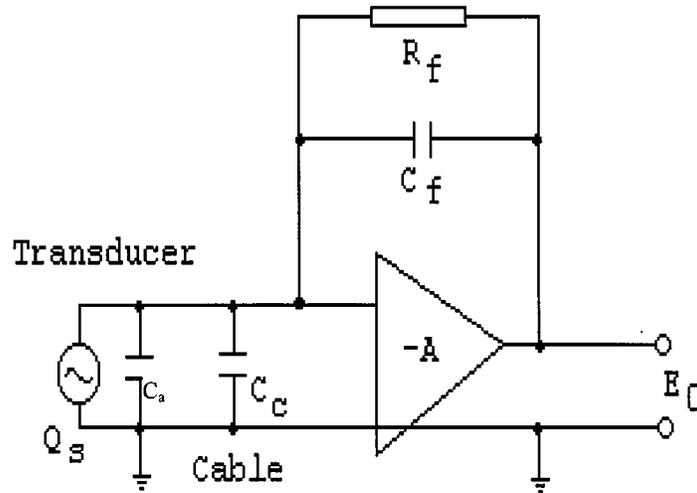
**FIGURE 17.20** A typical charge amplifier. The transducer charge, which is proportional to acceleration, is first converted to voltage form to be amplified. The output voltage is a function of the input charge. The response of the amplifier can be approximated by a first-order system. In PZT transducers, the preamplifier is integrated within the same casing.
