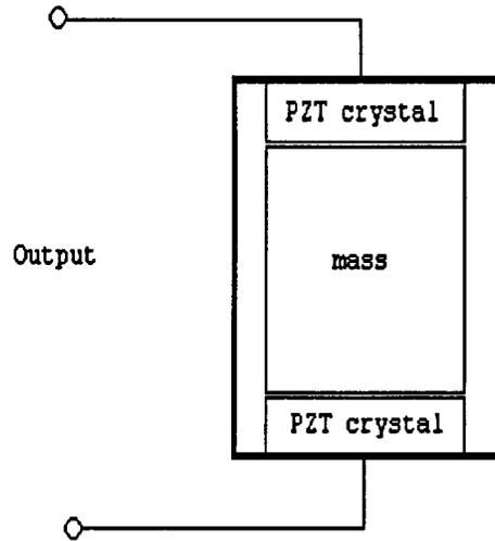
**FIGURE 17.8** A compression-type piezoelectric accelerometer. The crystals are under compression at all times, either by a mass or mass and spring arrangement. Acceleration causes a deformation of the crystal, thus producing a proportional electric signal. They are small in size and widely used. They demonstrate poor performance at low frequencies.
