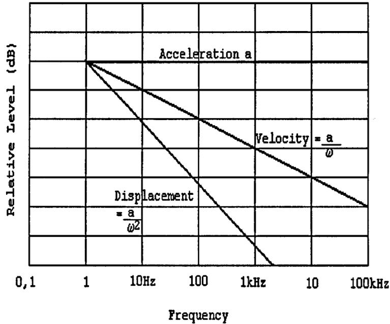
**FIGURE 17.2** Logarithmic relationship between acceleration, velocity, and displacement. Velocity at a particular frequency can be obtained by dividing acceleration by a factor proportional to frequency. For displacement, acceleration must be divided by a factor proportional to the square of the frequency. Phase angles need to be determined separately, but they can be neglected in time-averaged measurements.
