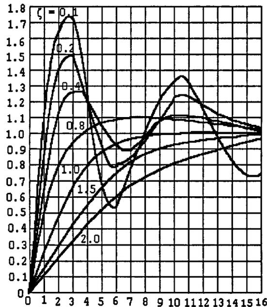
**FIGURE 17.4** Unit step time responses of a second-order system with various damping ratios. The maximum overshoot, delay, rise, settling times, and frequency of oscillations depend on the damping ratio. Smaller damping ratios give faster response but larger overshoot. In many applications, a damping ratio of 0.707 is preferred.
