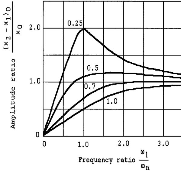
**FIGURE 17.13** A typical displacement of a seismic instrument. Amplitude becomes large at low damping ratios. The instrument constants should be selected such that, in measurements, the frequency of vibration is much higher than the natural frequency (e.g., greater than 2). Optimum results are obtained when the value of instrument constant  $c/c_c$  is about 0.7.
