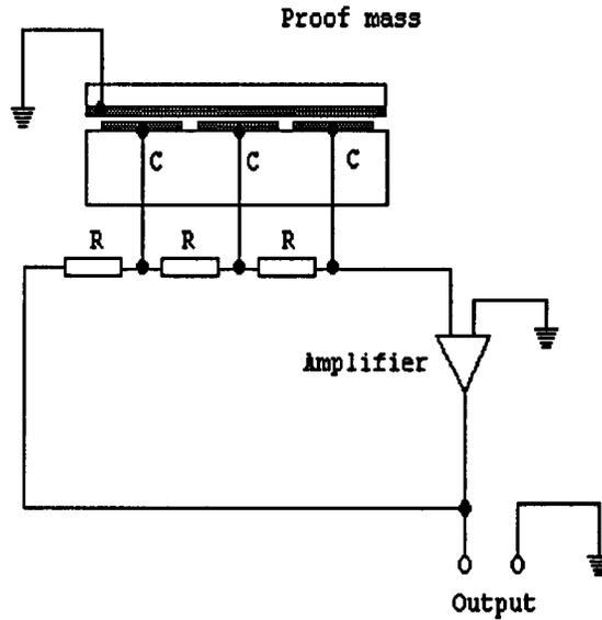
**FIGURE 17.11** A typical differential capacitive accelerometer. The proof mass is constrained in its null position by a spring. Under acceleration, variable frequencies are obtained in the electric circuit. In a slightly different version, the proof mass may be constrained by an electrostatic-feedback-force, thus resulting in convenient mechanical simplicity.
