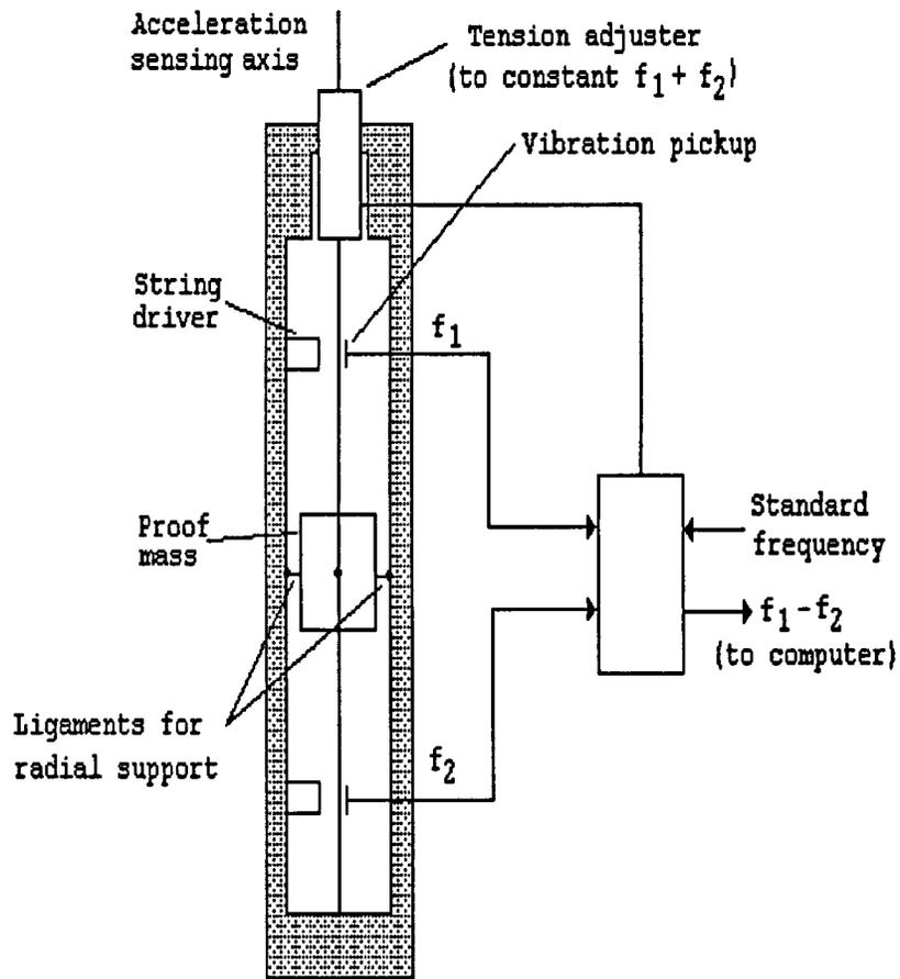
**FIGURE 17.16** A vibrating string accelerometer. A proof mass is attached to two strings of equal mass and length and supported radially by suitable bearings. The vibration frequencies of strings are dependent on the tension imposed by the acceleration of the system in the direction of the sensing axis.
