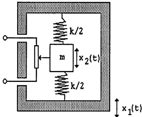
**FIGURE 17.14** A potentiometer accelerometer. The relative displacement of the seismic mass is sensed by a potentiometer arrangement. The potentiometer adds extra weight, making these accelerometers relatively heavier. Suitable liquids filling the frame can be used as damping elements. These accelerometers are used in low-frequency applications.
