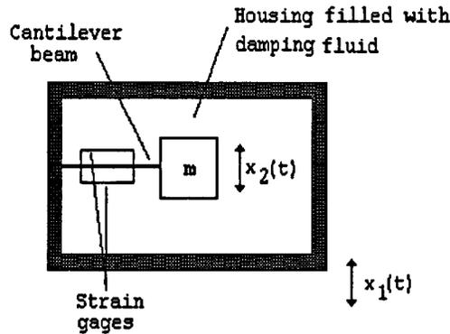
**FIGURE 17.15** A strain gage seismic instrument. The displacement of the proof mass is sensed by piezoresistive strain gages. The natural frequency of the system is low, due to the need of a long lever beam to accommodate strain gages. The signal is processed by bridge circuits.
