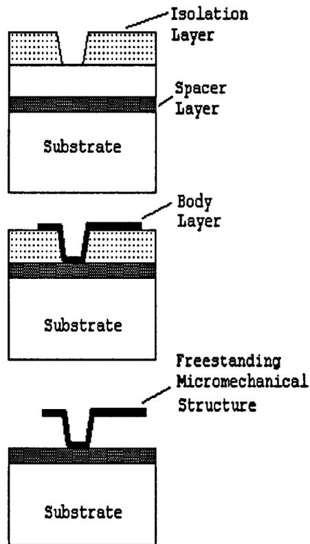
**FIGURE 17.17** Steps of surface micromachining. The acceleration-sensitive, three-dimensional structure is formed on a substrate and a sacrificial element. The sacrificial element is etched to leave a free-standing structure. The spacing between the structure and substrate is about  $2\ \mu\text{m}$ .
