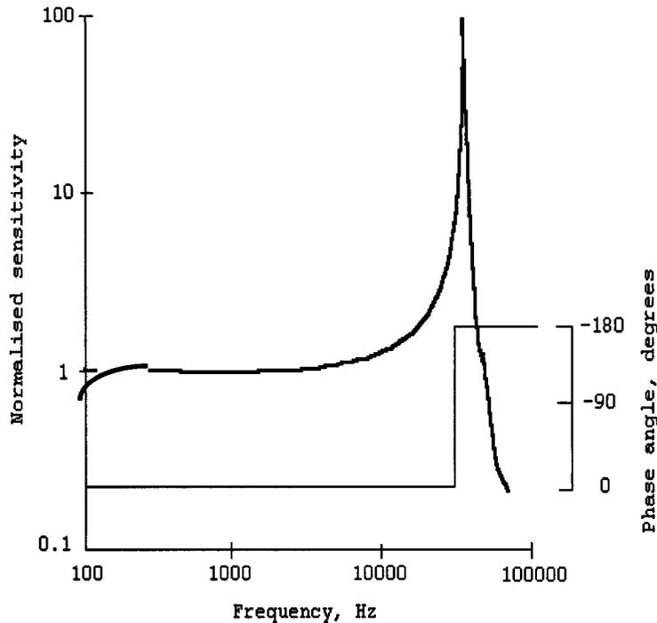
**FIGURE 17.9** Frequency response of a typical piezoelectric accelerometer. Measurements are normally confined to the linear portion of the response curve. The upper frequency of the accelerometer is limited by the resonance of the PZT crystal. The phase angle is constant up to the resonance frequency.
