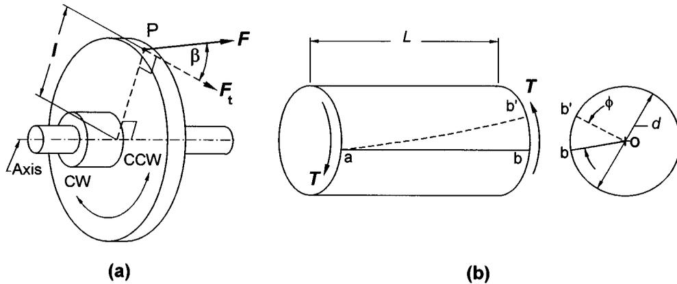
**FIGURE 24.1** (a) The off-axis force  $F$  at  $P$  produces a torque  $T = (F \cos \beta)l$  tending to rotate the body in the CW direction. (b) Transmitting torque  $T$  over length  $L$  twists the shaft through angle  $\phi$ .
