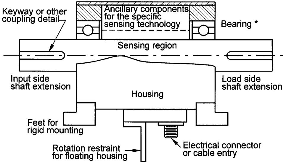
FIGURE 24.4 Modular torque transducer showing generic features and alternative arrangements for free floating or rigid mounting. Bearings\* are used only on rotational models. Shaft extensions have keyways or other features to facilitate torque coupling.
