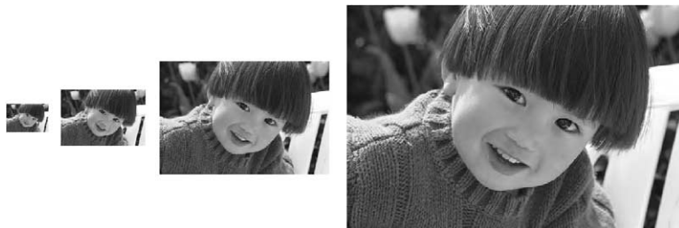
Fig. 19. Example of resolution progressive bit-stream ordering.
